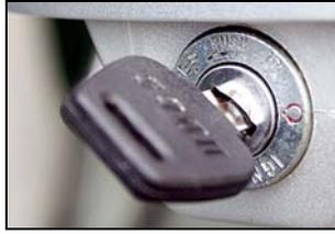
To release the battery turn the key in the battery to the open position – key aligns with symbol of a battery.
