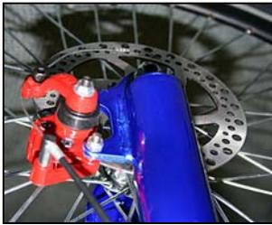
With the cycle upside down, adjust the front disc brake mechanism. Use an Allen key (or similar), to release, adjust and retighten the brake cable, until the wheel spins freely and the brake operates effectively when applied.
