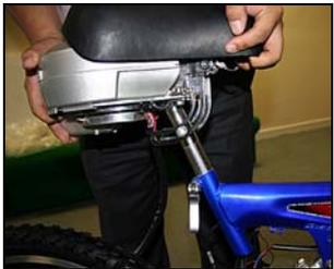
Insert the stem of the saddle and battery assembly into the frame. Align the saddle correctly with the frame and at the required height.
