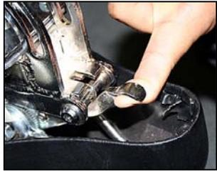
A lever under the seat releases a lock, allowing the seat to be lifted forward on a hinge, this makes the battery more accessible.
