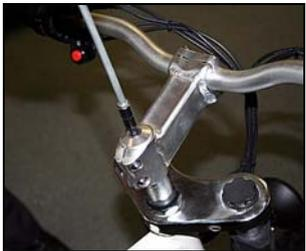
Align the handlebars with the rest of the bicycle, then use an Allen key or hexagonal tool to tighten them.
