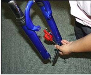
Remove the black plastic front fork protectors, which are part of the protective packing material.
