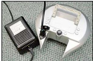
Open the cover on the battery socket and connect the charger connection plug. Plug the charger in to the mains supply and switch on. Charge indoors away from water and combustibles.
