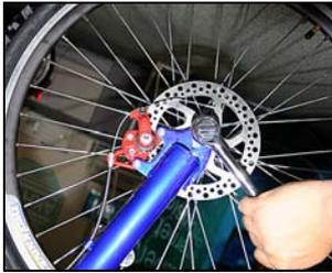
Place the wheel between the forks, ensuring that the brake disc is on the same side as the Brake Caliper (coloured Red).
