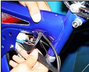
Once you have checked that the connections are correct, tidy the wiring by easing it into the gap in the frame, taking care not to break the connections.
