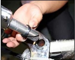
Insert the handlebar stem into the frame as shown.
