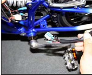
Join the electrical connectors from the frame to those from the battery housing.
