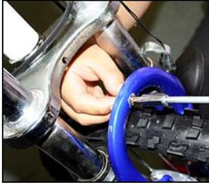
The front light is already secured to the frame via wires. Screw the front light bracket to the arch in front of the front fork, and then secure the light on the bracket.
