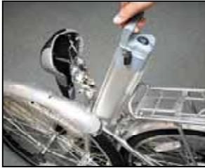
Slide the battery from the base housing.
