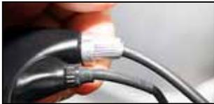
Fine adjustments to the brake tensions can be made via adjustment controls located at the junction of the brake lever and cable.
