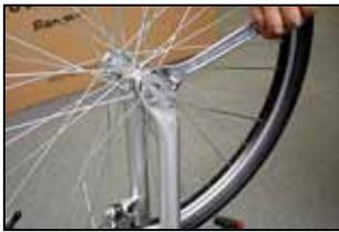
Use a spanner to secure the nuts firmly to the forks.
