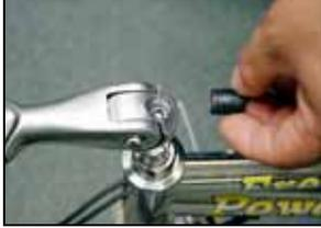
Remove the oval cover from the top of the handlebar stem. This will allow you to access the hexagonal handlebar adjustment slot.
