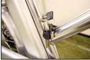
To release the battery, start by turning the key that is on the vertical tube.
