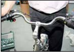
Align the handlebars 90 degrees to the forks.
