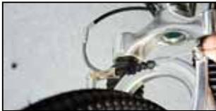
On the opposite side of the wheel, a nut is fixed to the brake mechanism, holding the wire cable. Loosen this nut to allow you to pull the cable through and take up any slack. Then re-tighten the nut. Check that the wheel spins freely and the brake operates effectively when applied.
