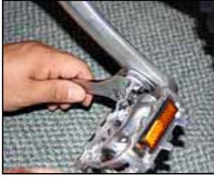
Pedals are marked L and R, for the left and right hand side of the bicycle when it is facing forward. Screw each pedal into the appropriate pedal shaft by hand, and then tighten with a spanner to secure.
