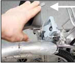
A lever under the seat releases a latch, allowing the seat to be lifted forward on a hinge, this makes the battery accessible.
