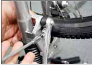
With the cycle upside down, ensure that the brake blocks have clearance from, and are parallel to the wheel rims. Use an Allen key or hexagonal tool to adjust and secure the blocks
