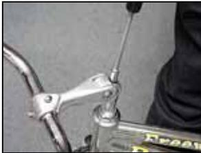
Finally, use an Allen key or hexagonal tool to tighten the handlebars in place.
