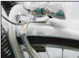
The mud guard and the front lamp support bracket share a nut and bolt attachment on the brake support arch.
