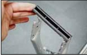
Remove the black plastic front fork protectors, which are part of the protective packing material.
