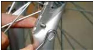
Attach the lower mud guard support struts to each side of the front wheel fork, using the nuts and bolts supplied.
