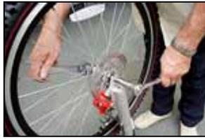
Use a spanner or socket set to tighten the outer nuts (outside the fork) so that the wheel is secured firmly to the fork.
