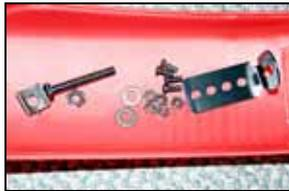
Small components for fixing mudguards
