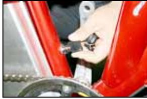
To remove the battery, turn the key on the vertical tube. The barrel will release, allowing the battery to be withdrawn.
