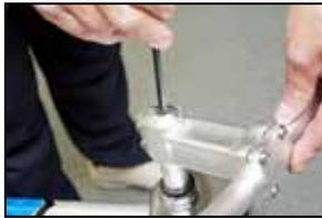
Finally, use an Allen key or hexagonal tool to tighten the handlebars in place.
