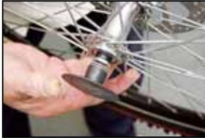
Remove the protective plastic nut from the wheel. This is part of the packing material.
