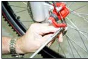
Use an Allen key to release the brake cable, and then pull it through to take up the slack. Tighten the Allen nut once the cable is tight and retest the brakes. Adjust the cable until the wheel turns freely and the brakes are effective.
