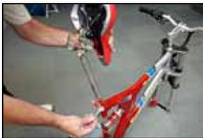
Insert the saddle stem into the frame. Use the lever clip to secure the saddle in place. If the clip is too loose or too tight, adjust the lever in relation to its opposing nut to achieve a firm closure.
