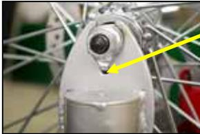
Insert the lock washer into the small hole in the fork.
