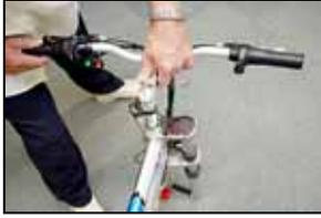
Align the handlebars 90 degrees to the forks.
