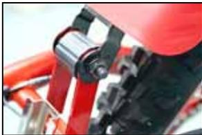
**REAR** Fix the rear mudguard directly to the support bracket that is integral to the frame. Insert the plastic barrel between the integral frame supports. Place the mudguard supports on the outside edges of the frame supports and tighten the nut and bolt.
