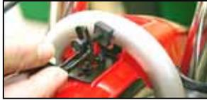
Attach the mudguard bracket and the front light bracket to the arch (the front light is already connected to the bike by its wires).
