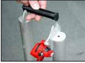
Remove the black plastic front fork protectors, which are part of the protective packing material.
