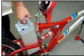
Using the handle provided, pull upward to slide the battery from the base housing.
